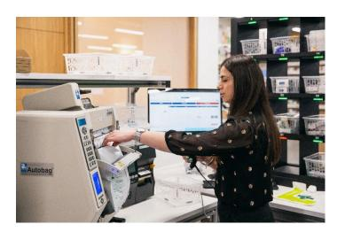
In a FLOWRx Hub Manual, packs are scanned from the FLOW Tote to print a patient label, the label is affixed to the pack and scanned again. On this scan the RFID LED Smart Shelves guide the operator to sort the right medication into patientspecific baskets. You can then choose to automate the bagging or packing of medication by patient or leave this as a manual process too. Our software will then use barcode technology to sort patient medication bags into store specific totes.
